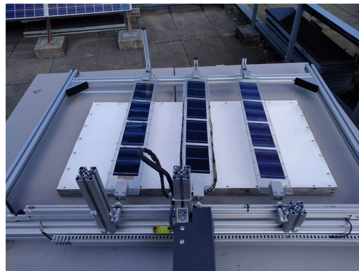
Miniaturized test array. The arrangement is the downscaled version of the large test array shown above.
