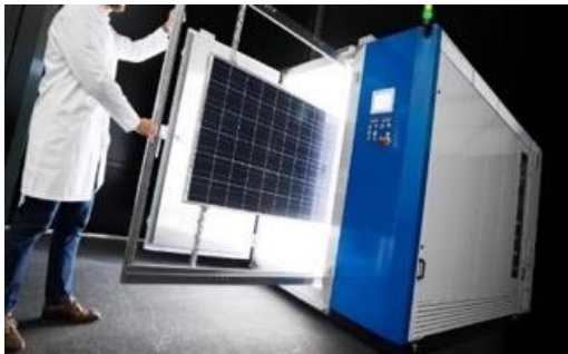
Steady State AAA+ Sun Simulators Integrated in Climate Chambers
