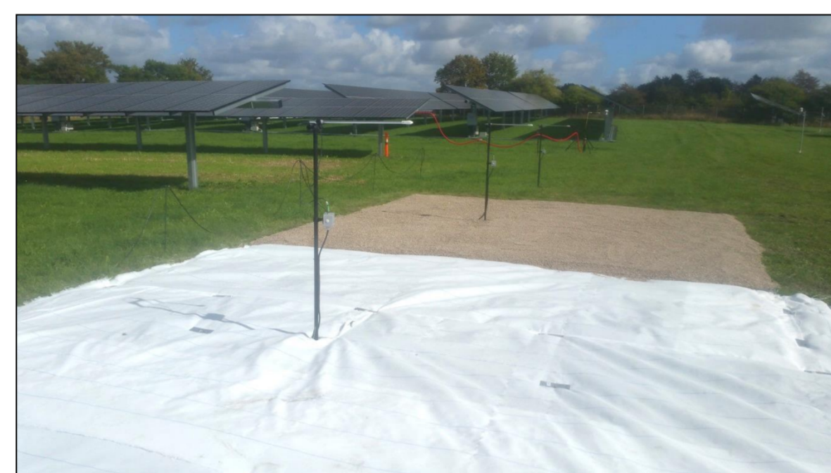
Broadband albedo data from the unshaded measurement zones are used as input to bifacial PV performance models.
