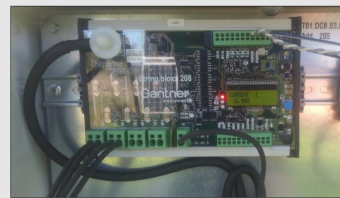
DC Power meters with isolated surface mount resistors and digital filtering
