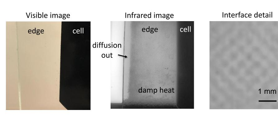
Sample: One cell mini-module fabricated with Solite double glass, ethylene vinyl acetate encapsulant, interdigitated back contact cell (SunPower)
