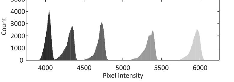
**Quantitative imaging.** Upper panel: transmission bandpass images of a polyimide film equilibrated at 10, 30, 50, 70 and 90% relative humidity and 30 °C, showing an increase in intensity with lower water content. Lower panel: pixel intensity histogram of the same images. Imaging can be correlated with the independently measured absolute water content with linear or higher order interpolation.
