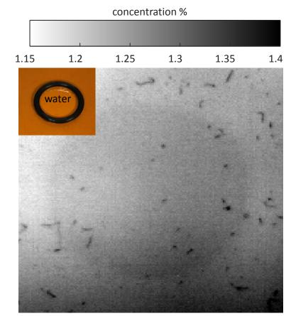
Hydroscanner instrumentation. Development of a novel infrared imaging technique to determine water content in polymers. Applicability in testing photovoltaic module packaging materials and imaging through white backsheet for indicators of degradation: corrosion, cracking and delamination.
