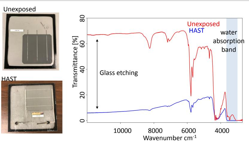
Sample: One cell mini-module fabricated with Solite glass, ethylene vinyl acetate encapsulant, architectural glass, and edge seal Accelerated testing: HAST (highly accelerated stress testing, 120 °C, 10 psi pressure, 100% relative humidity) for 500 hours Spectroscopic testing through clear sections of the mini-module
