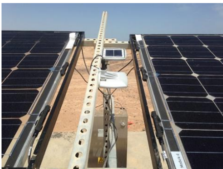
Irradiance sensors front and rear in the plane of the module
