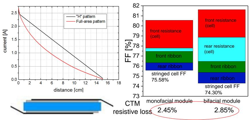
Current flow pattern is different for monofacial and bifacial cells
