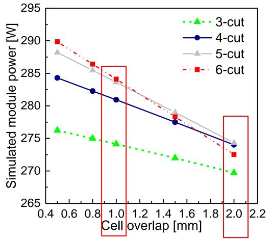
Number of cell cuts is limited by throughput and cutting losses.
