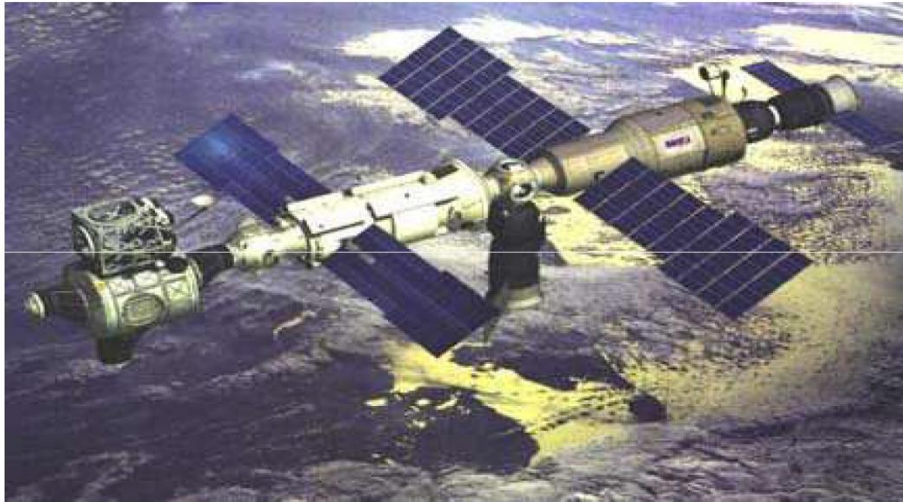
Bifacial Si solar arrays were mounted on spacecrafts "Zarya" and "Zvezda" of Russian segment of the ISS.
