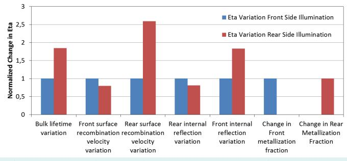
PC1D simulation of impact of parameter variations on front and rear efficiency
