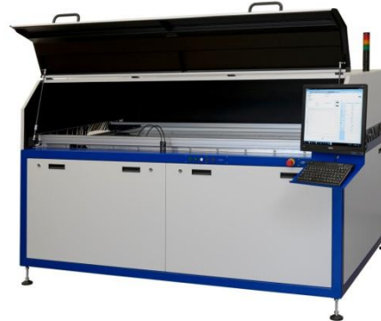
Pasan's Module Inspection System, MIS, and its bifacial-compatible black hood
