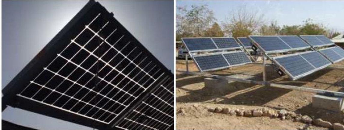
Test site in the Eilat-Eilot Desert, Israel, supervised by the Arava Outdoor PV Validation Lab, Eilat-Eilot, Israel (70 cm height above ground, 50% ground reflectance) Results (*): 17.2% bifaciality gain vs. German modules, 21.7% cell equivalent efficiency
