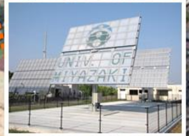
CPV 10 kW × 2 systems Sumitomo Electric Industries, Ltd.
