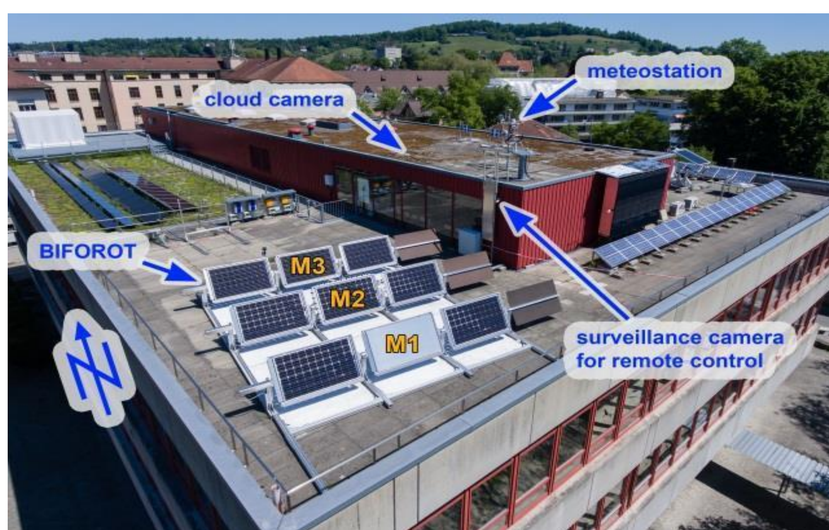
Biforot test rig in permanent rotation, 12 tilt angles from 0° to 90° every 1 minute
