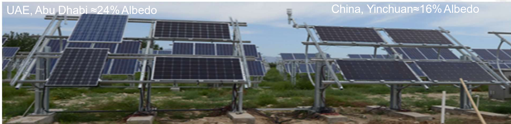
Albedo_POA (POAA): average albedo measured in tilt of module with silicon sensors.
